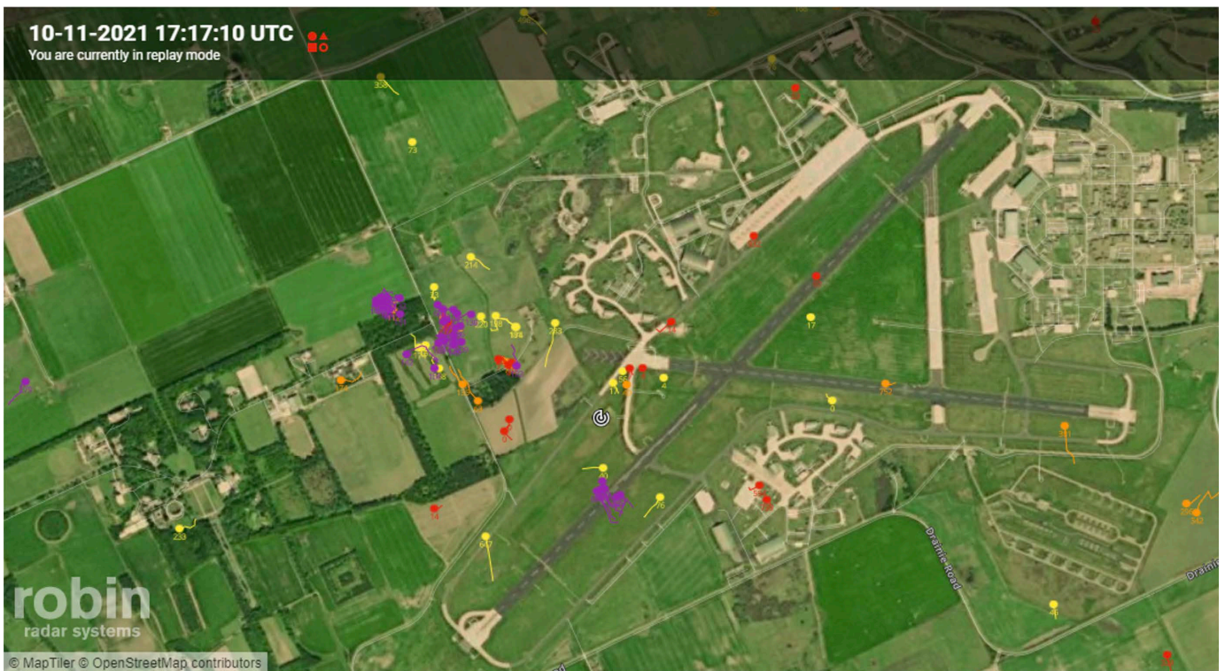
17:17 A second return shows high bird activity further up the cable and crossing the runway from SSE-NNW. Approximate height 600 - 1000ft.
